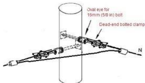
Figure 6 Dead-end corner (81 deg to 90 deg)
